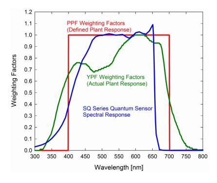
Radiation weighting factors for PPFD (defined plant response to radiation), YPFD (measured plant response to radiation), and Apogee SQ Series quantum sensors (sensor sensitivity to different wavelengths of radiation).
