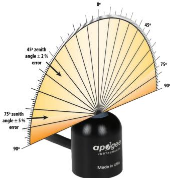
Directional, or cosine, response is defined as the measurement error at a specific angle of radiation incidence. Error for Apogee SQ series quantum sensors is approximately  $\pm$  2 % and  $\pm$  5 % at solar zenith angles of 45° and 75°, respectively.
