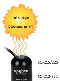
Example of PPFD measurement with an Apogee quantum sensor. Full sunlight yields a PPFD on a horizontal plane at the Earth's surface of approximately 2000  $\mu mol~m^{-2}~s^{-1}$ . This yields an output signal of 4000 mV for the 0-5 V option or an output signal of 2000 mV for the 0-2.5 V option. The signal is converted to PPFD by multiplying by the calibration factor.
